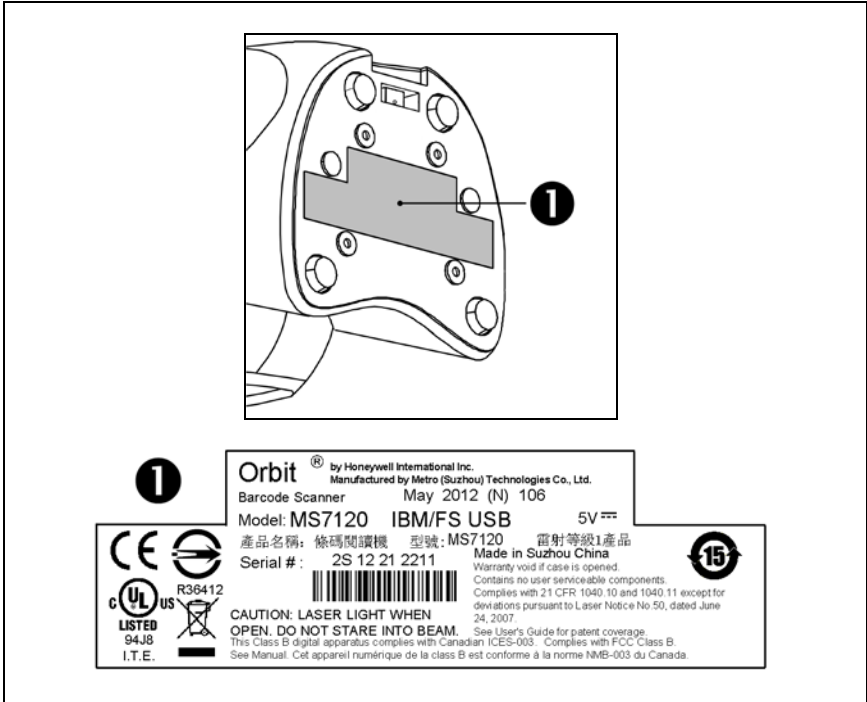
Figure 3. Labeling Locations on the Bottom of the Scanner and Examples
